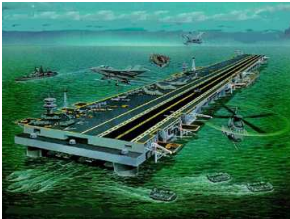
Figure 3.1 Mobile Offshore Base
